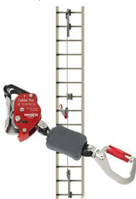
A permanent vertical fall protection system for often accessed structures such as ladders, towers or tanks that allows the worker to move up and down the entire height of the system rather than having to disconnect and find new tie-off points along the way.
